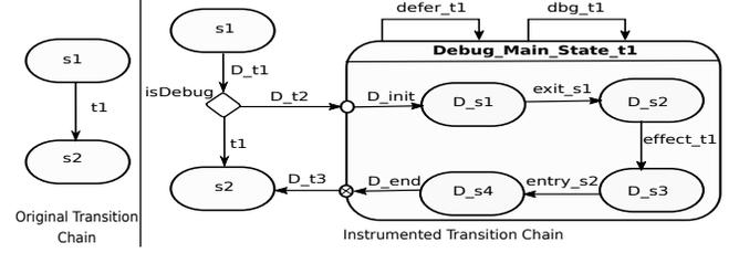
Figure 4: Model Instrumentation Overview
